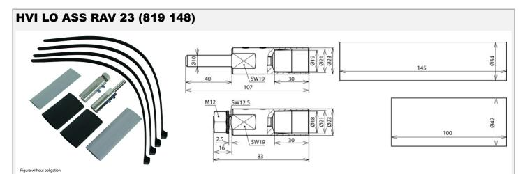
Connection elements for sealing the HVI long Conductor at both ends when implementing the sealing end of the conductor outside the supporting tube (head piece for connection plate) and connection element for connecting to other parts of the external lightning protection or earth-termination system (incl. four heat shrinkable sleeves and four cable ties).
